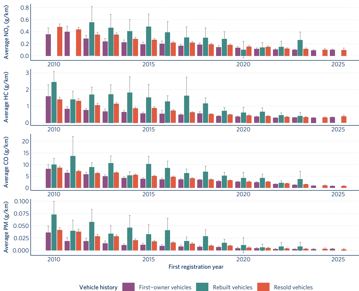
Figure 10. Petrol passenger car average NO x , HC, CO, and PM distance-specific emissions by first registration year and vehicle history
