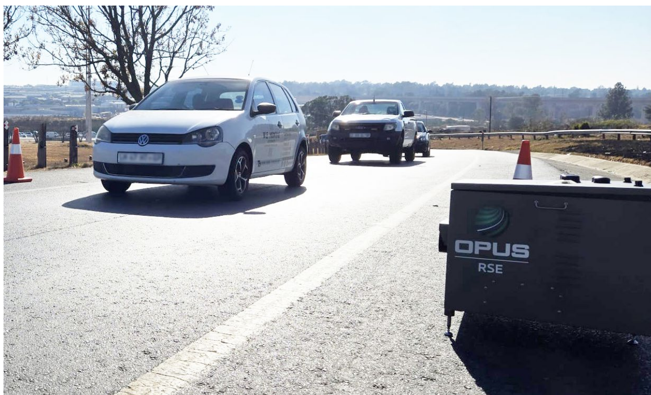
Figure 2. Remote sensing data collection using Opus RSD6000
