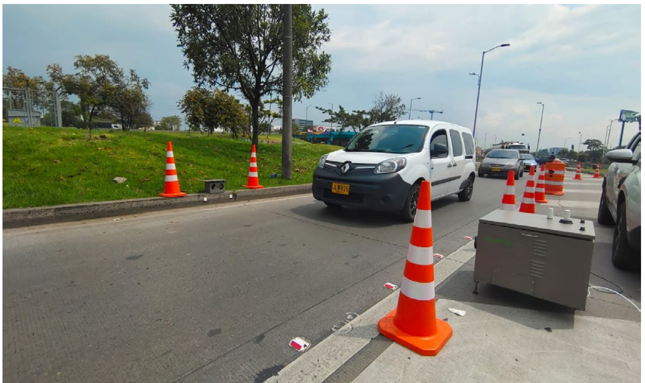
Figure 2. Remote sensing data collection using an Opus portable RSD5700 instrument
