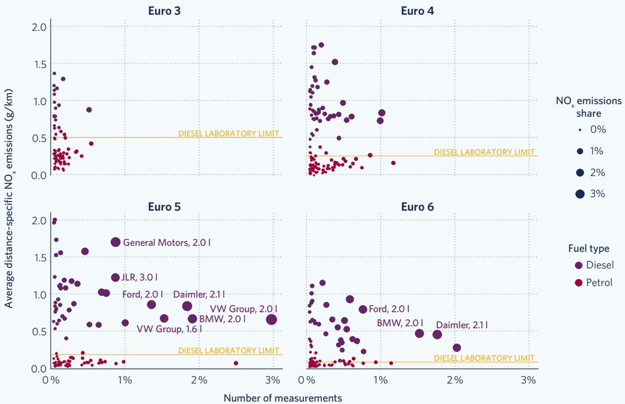
**Figure 15.** Average distance-specific NO<sub>x</sub> emissions and share of remote sensing measurements for each vehicle family measured in London in 2017–2018.
