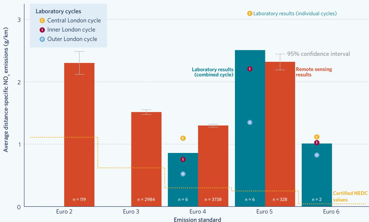
**Figure 12.** Distance-specific NO<sub>x</sub> emissions from diesel-fueled London taxis by Euro standard measured in the laboratory and by remote sensing.
