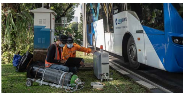
Figure 3. Remote sensing equipment set up at TransJakarta BRT dedicated lane.
