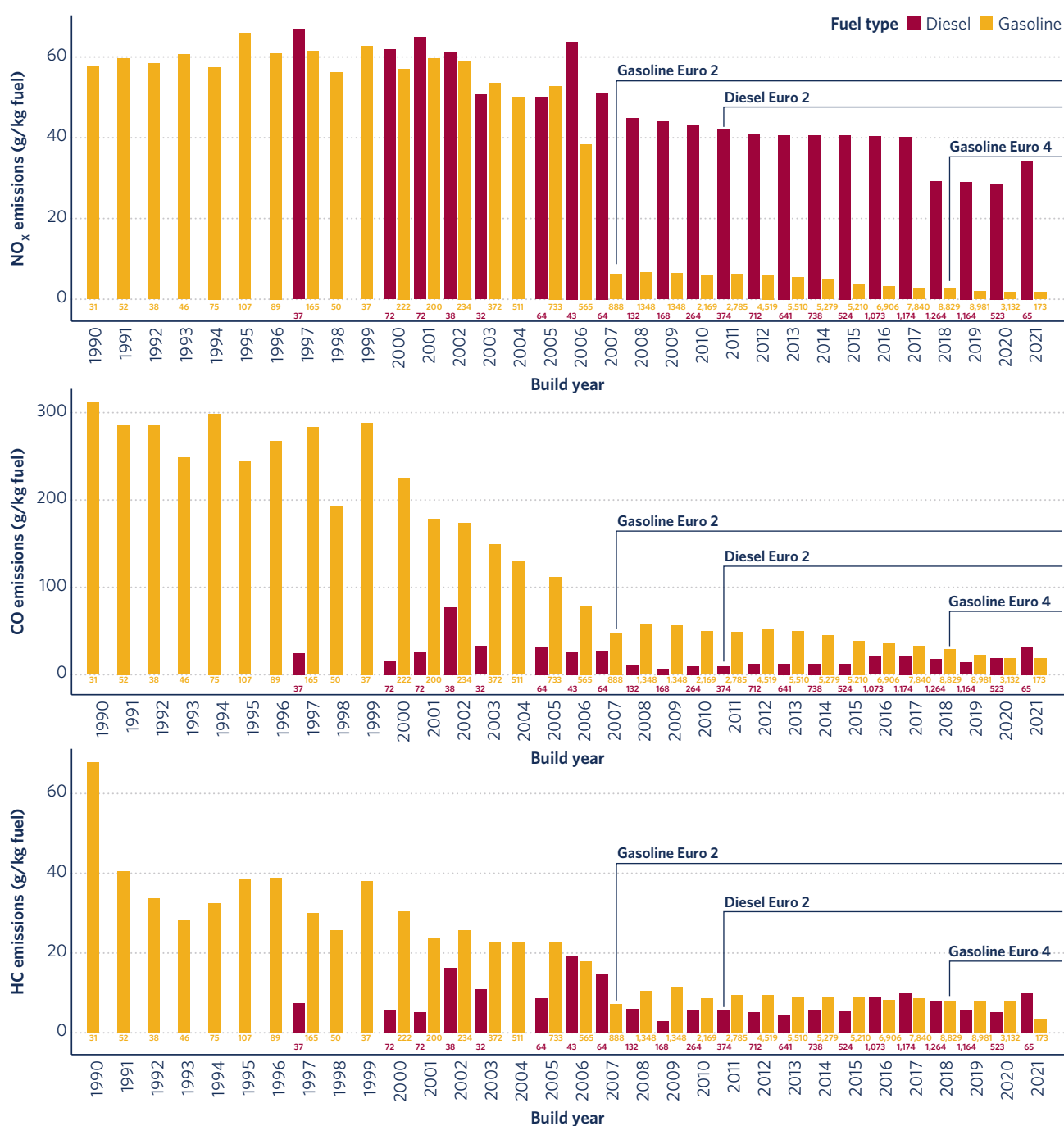
Figure 10. Median NO x , CO, and HC emissions of passenger vehicles by fuel type and build year.
