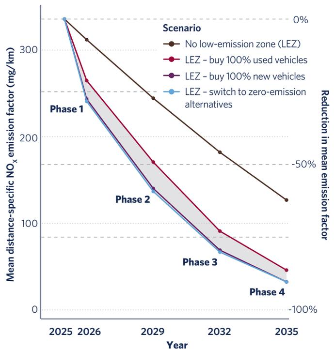
Figure 3. LEZ effects on fleet-average distance-specific  $\text{NO}_x$  emissions for passenger cars for four scenarios
