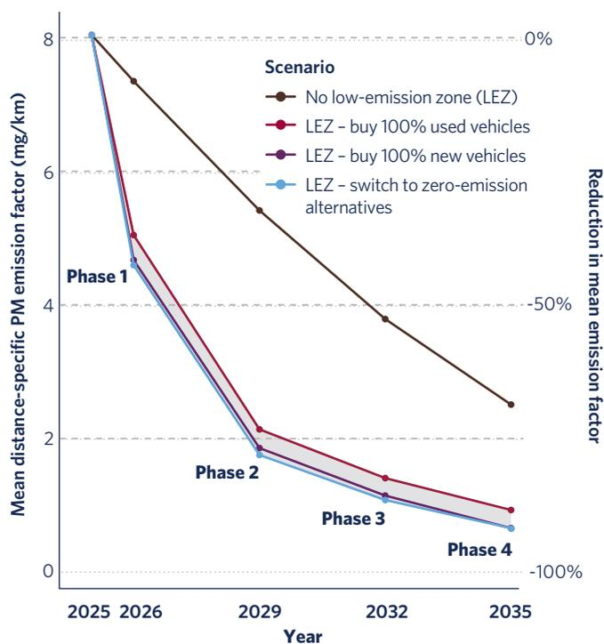
**Figure 4.** LEZ effects on fleet-average distance-specific PM emissions for passenger cars for four scenarios
