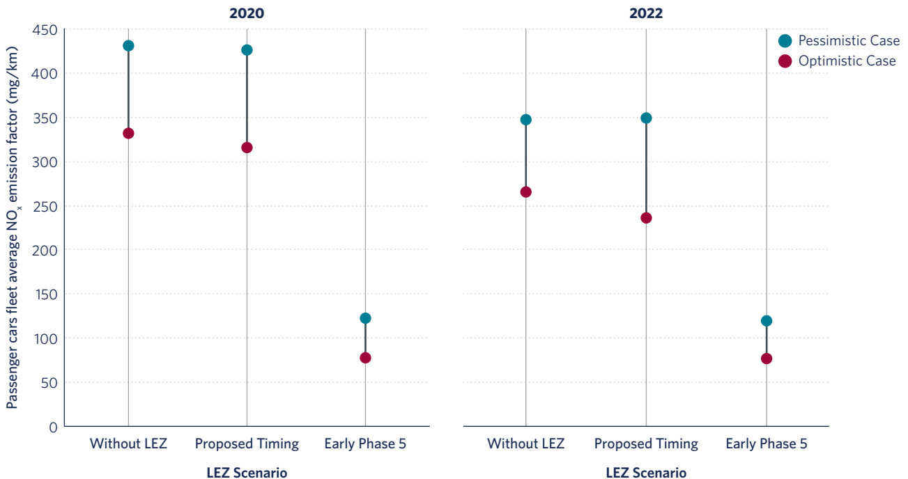
Passenger car fleet-average \text{NO}_x emission factor in 2020 and 2022 without the LEZ, with the proposed LEZ, and with earlier implementation of Phase 5.
